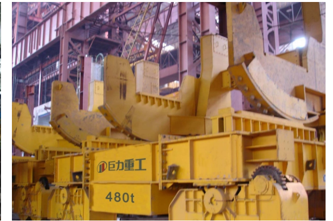
480t钢包车驱动 480t Buggy Ladle Drive
