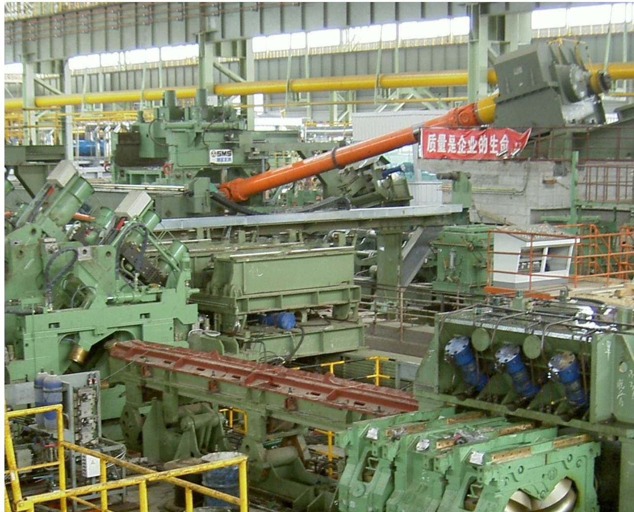
攀成钢无缝钢管机组 Pangang Group Chengdu Steel & Vanadium Co.,Ltd.Seamless Steel Pipe Unit
